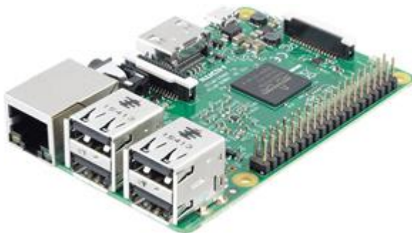
Fig. 6 Raspberry Pi model 3
